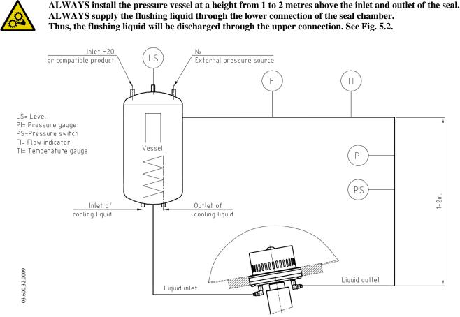
Figure 5.2 Pressure vessel installation scheme
